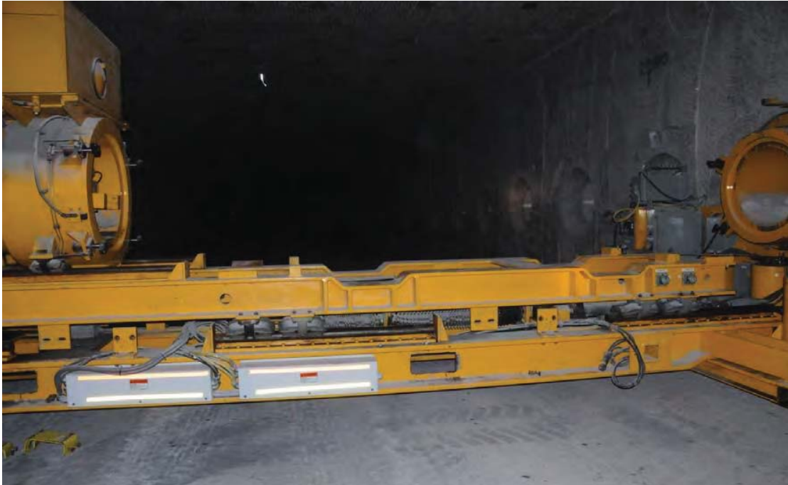
Figure 4 Equipment prepared for RH waste emplacement
