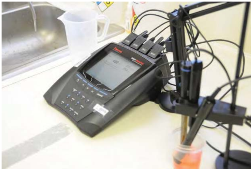
Figure 4. Calibration of pH Probe Using Orion 93 VersaStar Meter.
