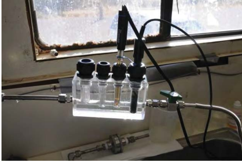
Figure 3. In-line Flow Sampling Cell Used To Measure the Field Parameter pH, Specific Conductance, and Temperature
