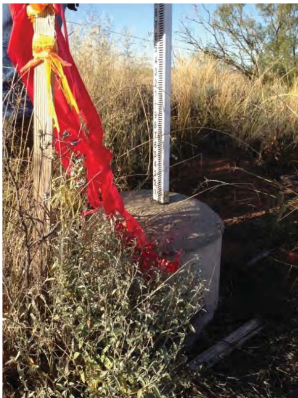
Figure 6. Surveying Rod on Monument S-24
